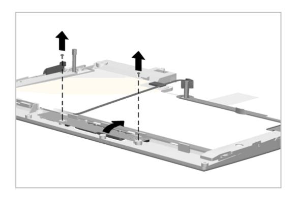
Figure 5-40. Removing the EasyPoint II Controller
